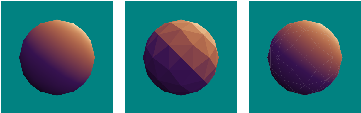
Figure 22: Images of mesh output for the sphere with a low sample resolution, using a body-centered arrangement with the integrated clustering algorithm. Flat shading is shown in the center, with the wireframe shown on the right.
