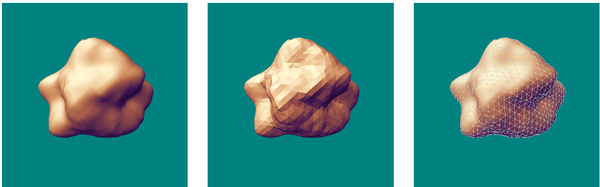
Figure 23: Images of mesh output for the asteroid with a medium sample resolution, using a body-centered arrangement with the integrated clustering algorithm. Flat shading is shown in the center, with the wireframe shown on the right.
